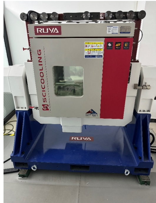
Figure 10: 2-axis incubator rate table
