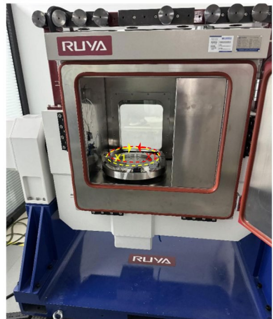
Figure 5: 2-axis incubator rate table
