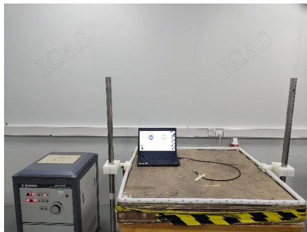
Power Frequency Magnetic Field Test Set-up
