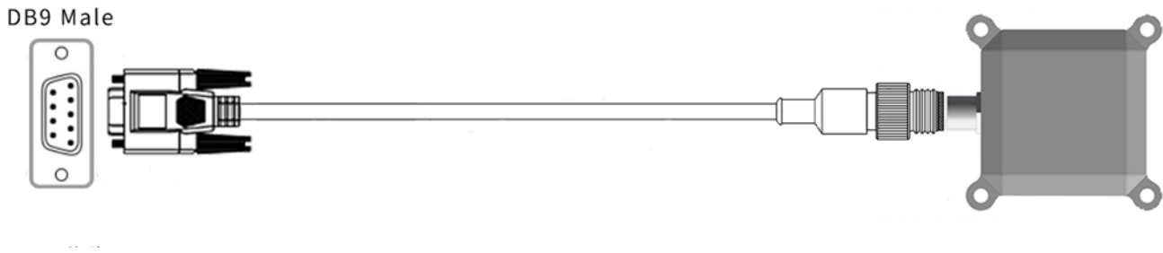
Figure 12: M8-A code 6 pin to DB9 internal power
